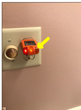
The receptacle has reverse polarity.
