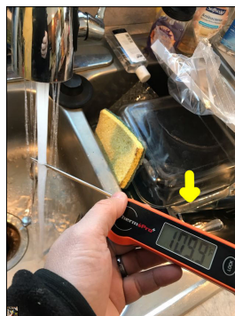
Temperature reading of the hot water during the time of the inspection. The approximate temperature of the hot water was 109 degrees Fahrenheit.
